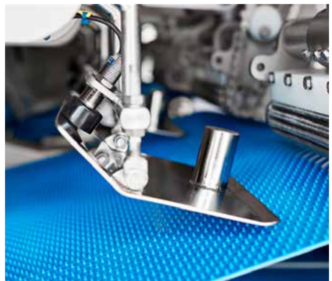
The active tail system ensures that the rollers will elevate before reaching the end of the tail.
